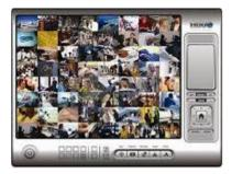
The system use 2 set high performances PC to manage all cameras. The PC configuration at least is Intel Dual Core i5 / i7 CPU, 2G RAM, 2G Graphic Card, 1000M Ethernet Interface. The video software management software on the computer can add, grouping, edit, delete, monitor, update all cameras and NVRs, use can monitor the 1/4/9/16/25/36ch video on the one screen, and also can divide all camera into many groups, for example 16ch per group, then can switch it one by one.
